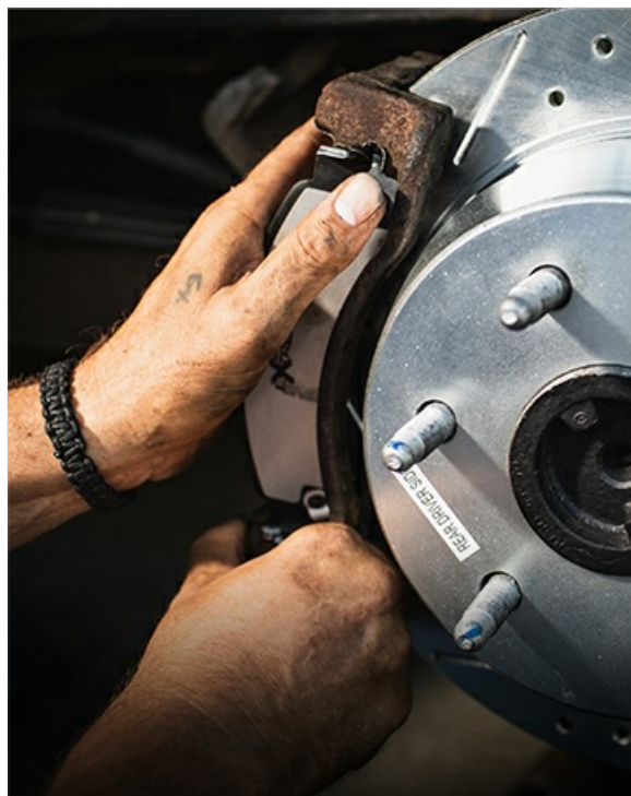
Figure 3.1: Hands installing new brake pads into a vehicle's caliper assembly.
