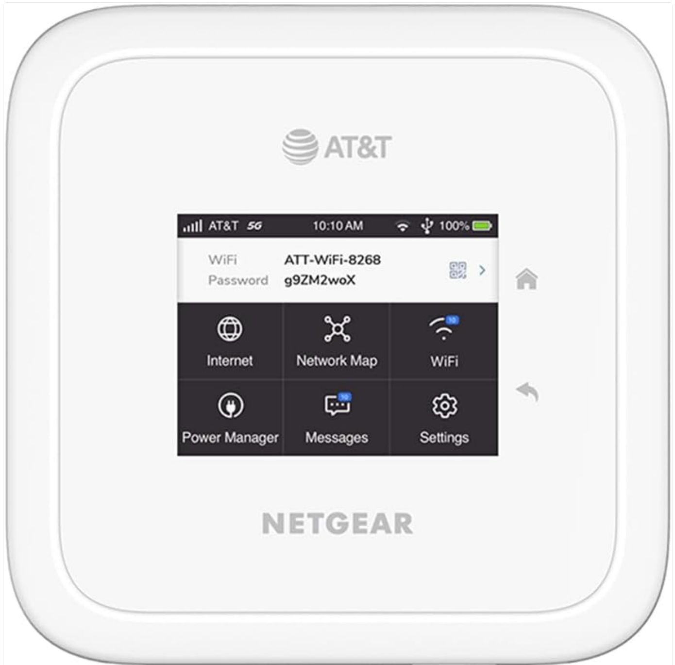
Figure 3: Front view of the NETGEAR Nighthawk M6, displaying the touchscreen with Wi-Fi SSID, password, and main menu icons.
