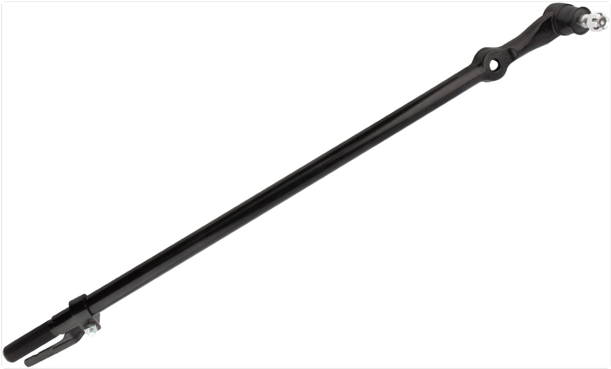
Image: The BOXI Front Center Drag Link, showing the adjustment sleeve and clamp mechanism. This part allows for length adjustment, which is critical for proper wheel alignment after installation.
