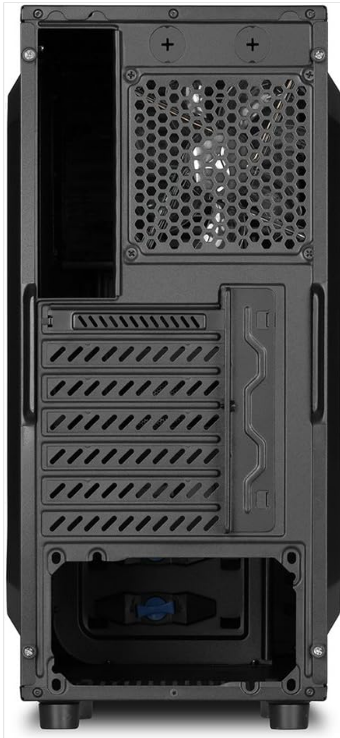
Figure 2.4: Rear view of the PC case, showing expansion slots and power supply mounting area.
