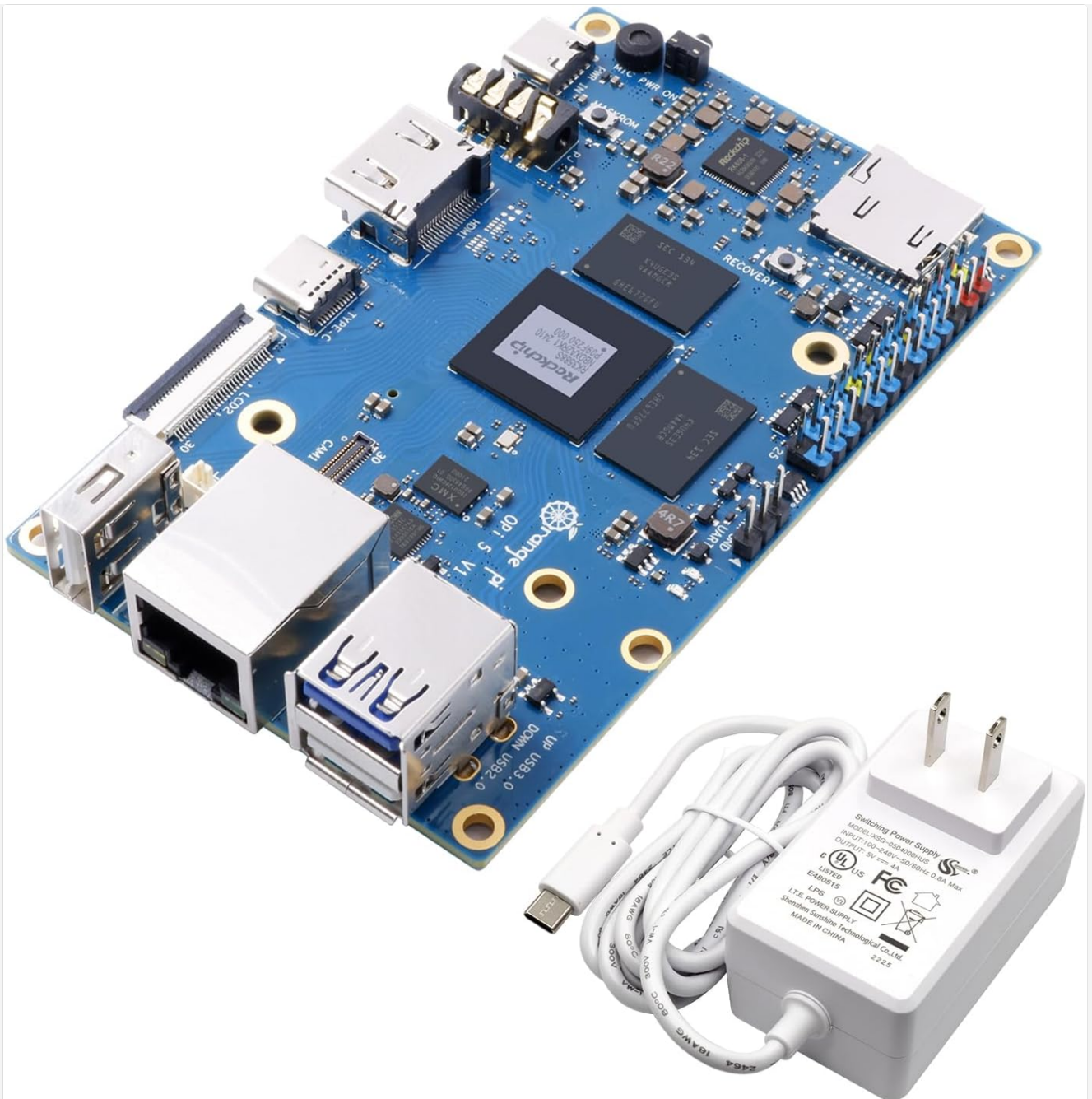
Figure 1: Orange Pi 5 4GB Single Board Computer and included 5V4A Type-C power supply.
