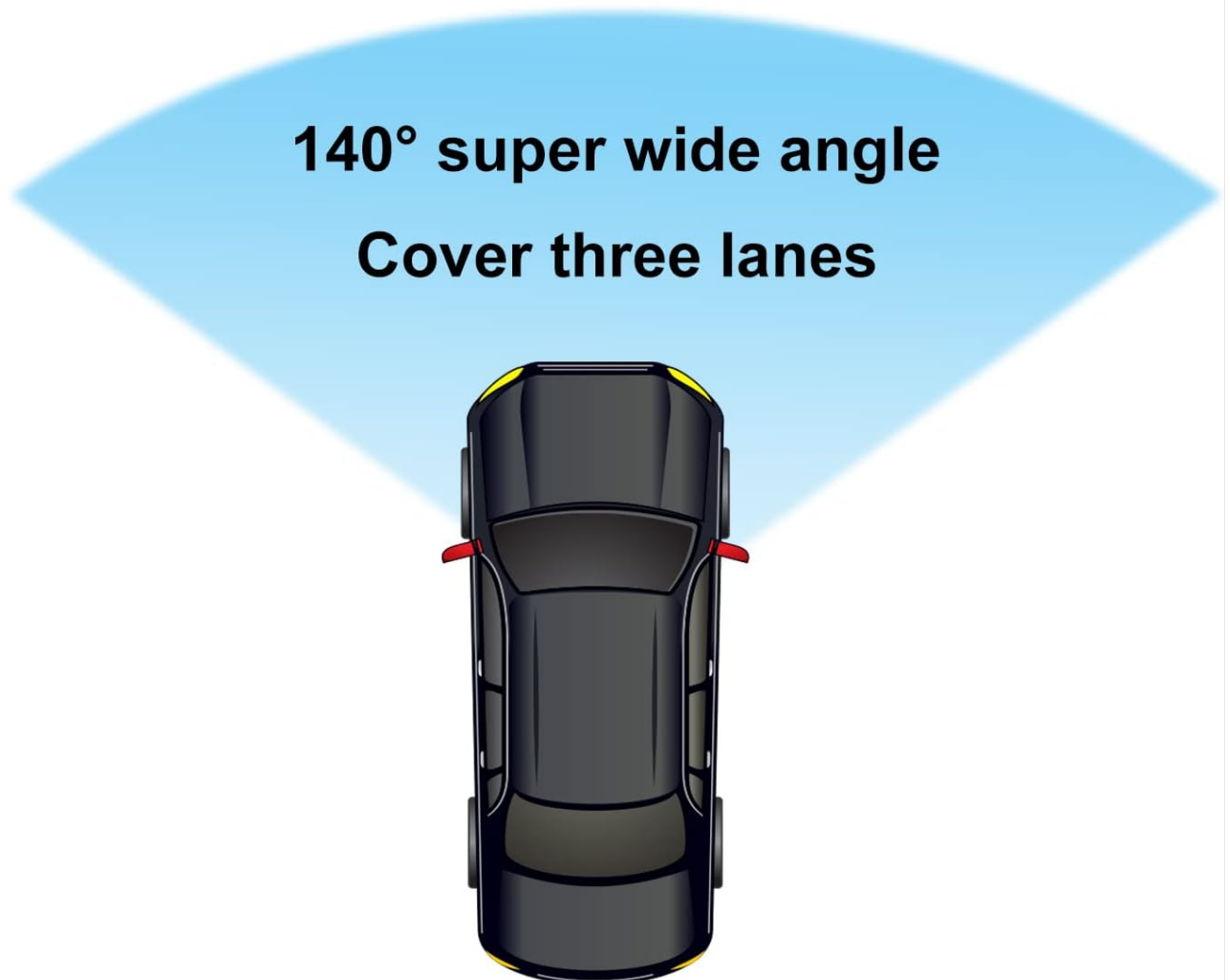
Figure 5.4: 140° wide viewing angle. This diagram shows a car from above with a blue fan-shaped overlay indicating a 140-degree super wide angle that covers three lanes.
