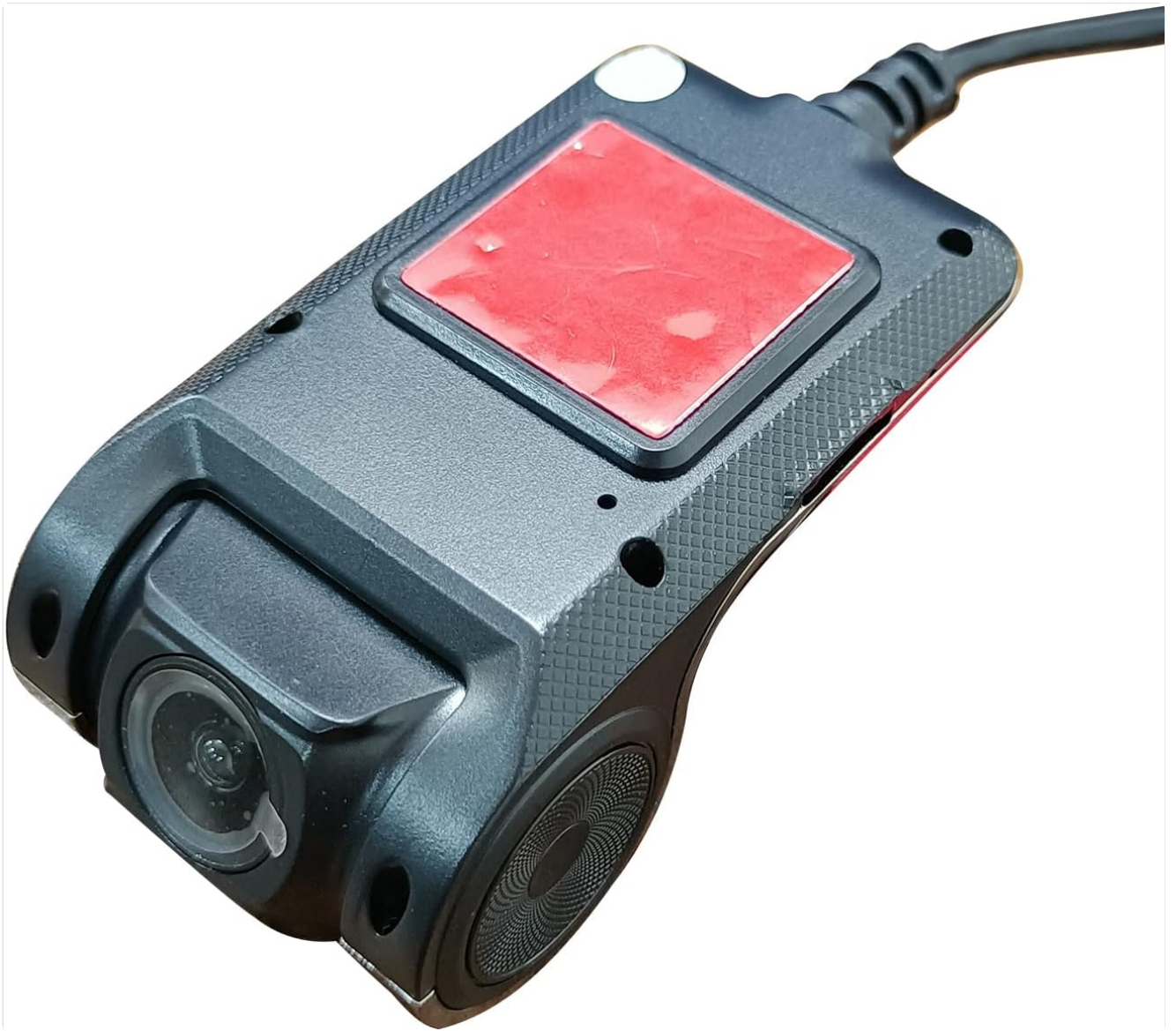
Figure 4.4: Pioowirk Car DVR showing the 3M adhesive pad on its top surface, used for mounting.
