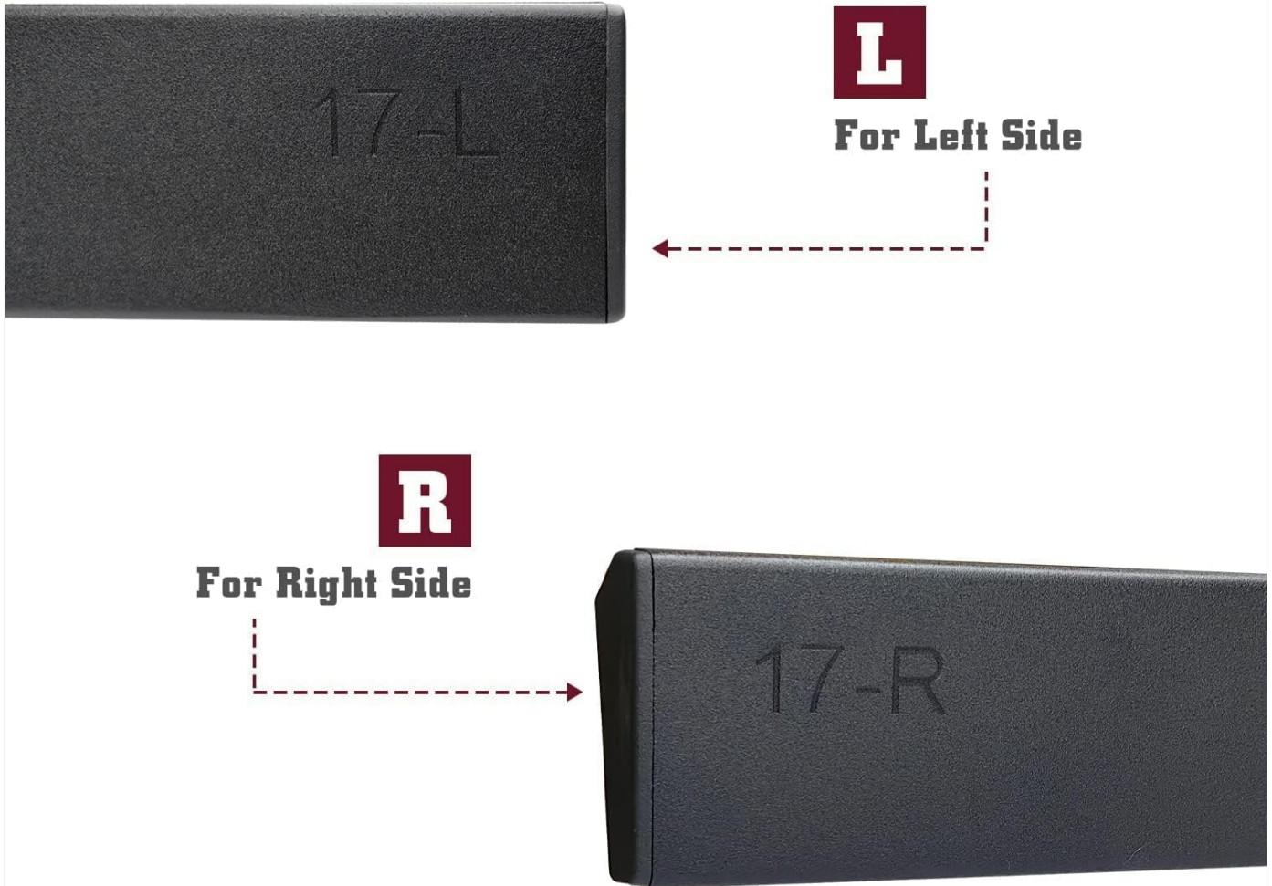
Image 5.1: Left and Right Bar Identification. This image demonstrates how to identify the correct side for each running board by checking the 'L' (Left) or 'R' (Right) marking on the front end of the step bar.
