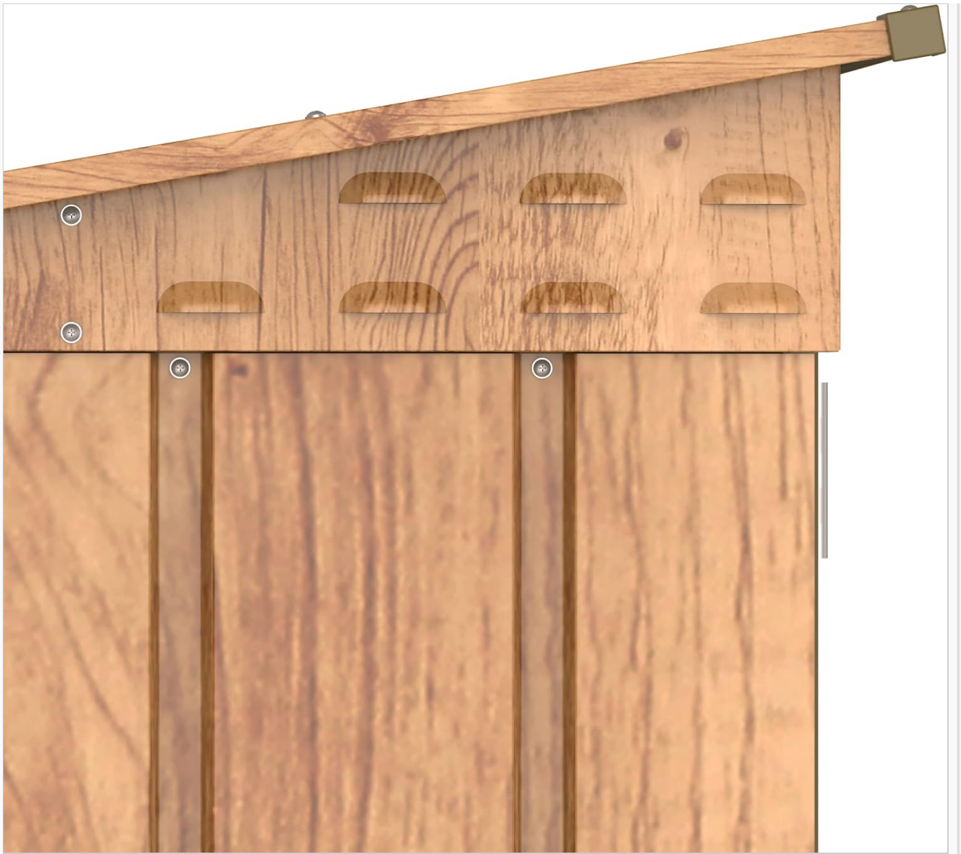
Figure 2.6: Close-up of the side panel, illustrating the integrated air ventilation system for improved circulation.
