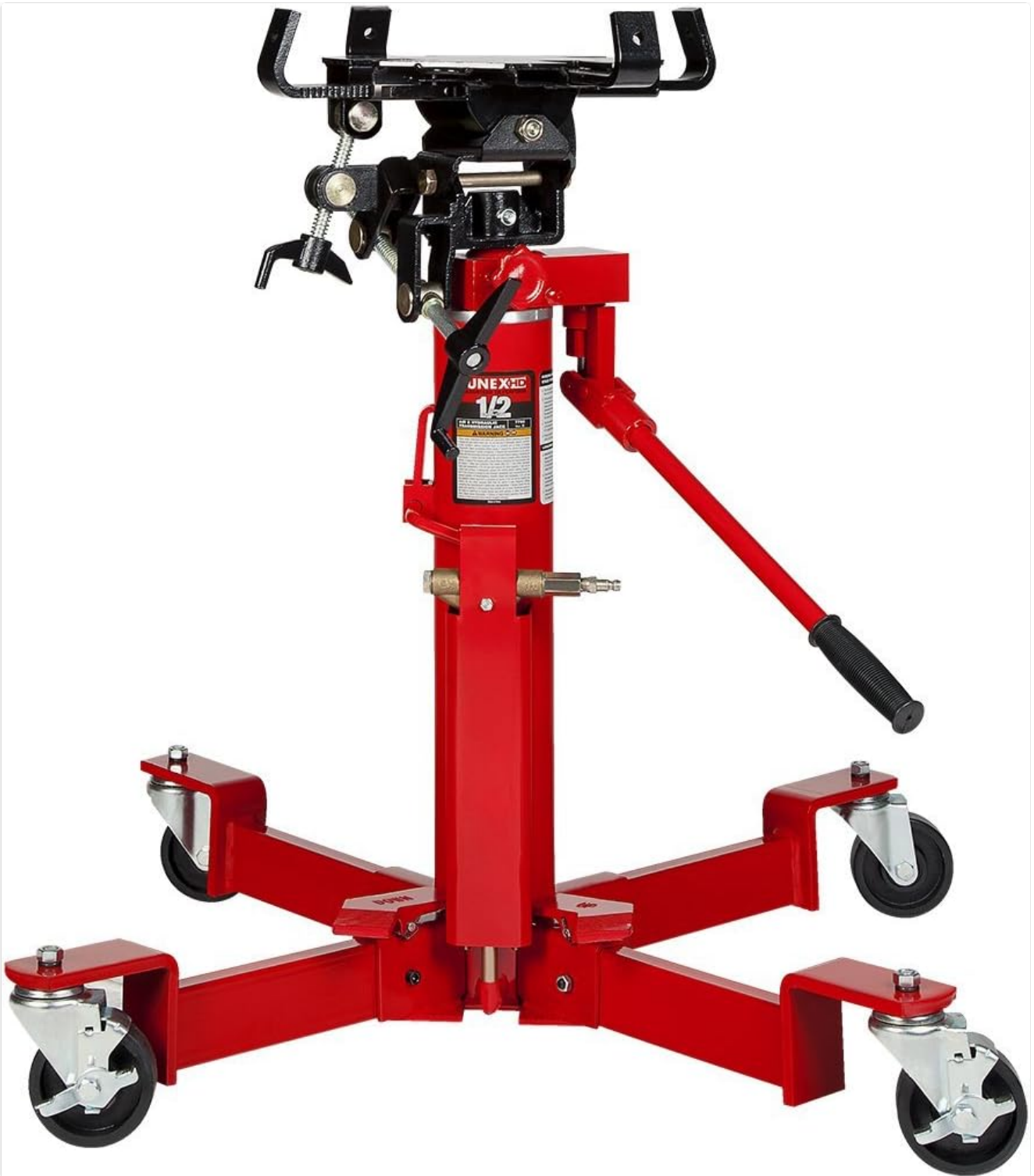
Figure 3.1: The Sunex 7796 Transmission Jack, showing its main components.
