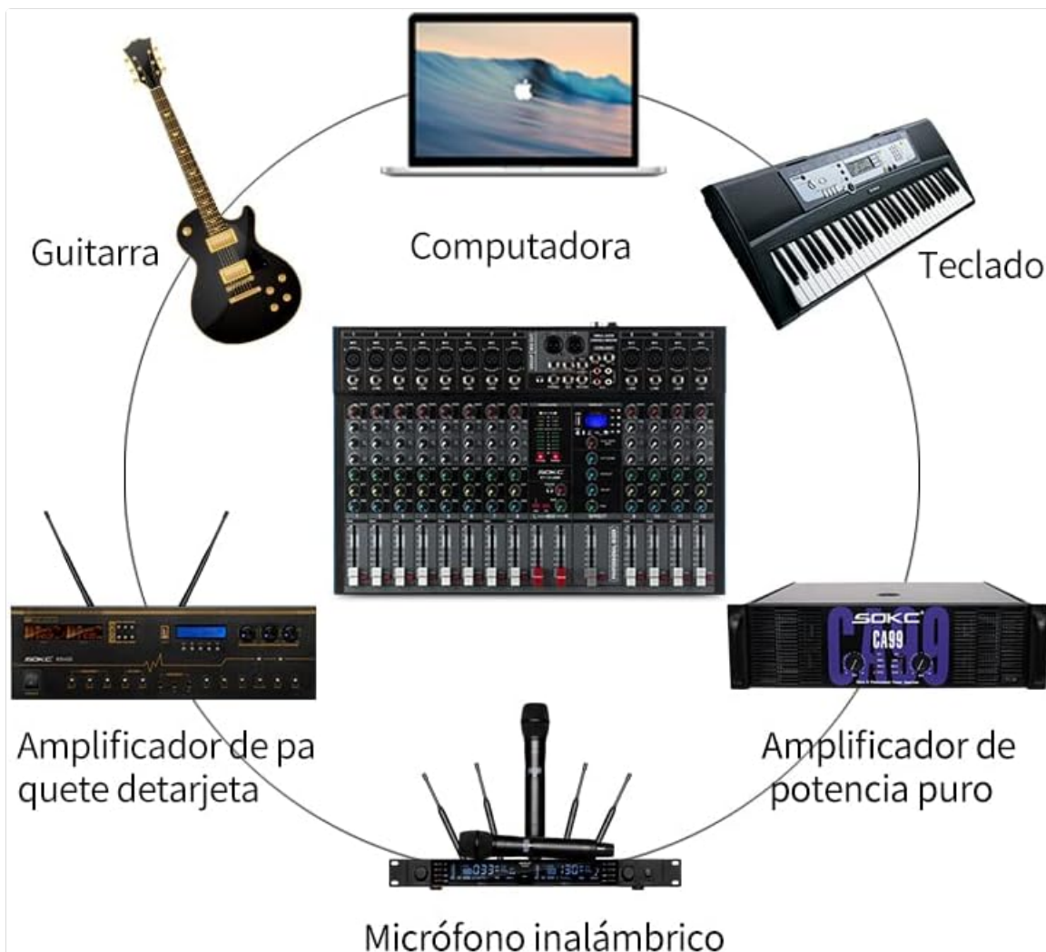
Figure 3.1: Example connection diagram for the ET12 mixer with various input and output devices.
