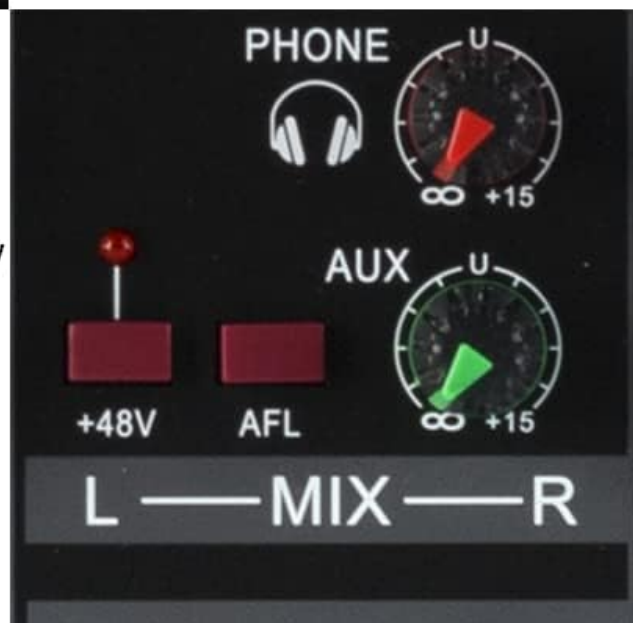
Figure 2.2: Detail of microphone (XLR) and line (1/4 inch) inputs, along with the +48V phantom power switch.
