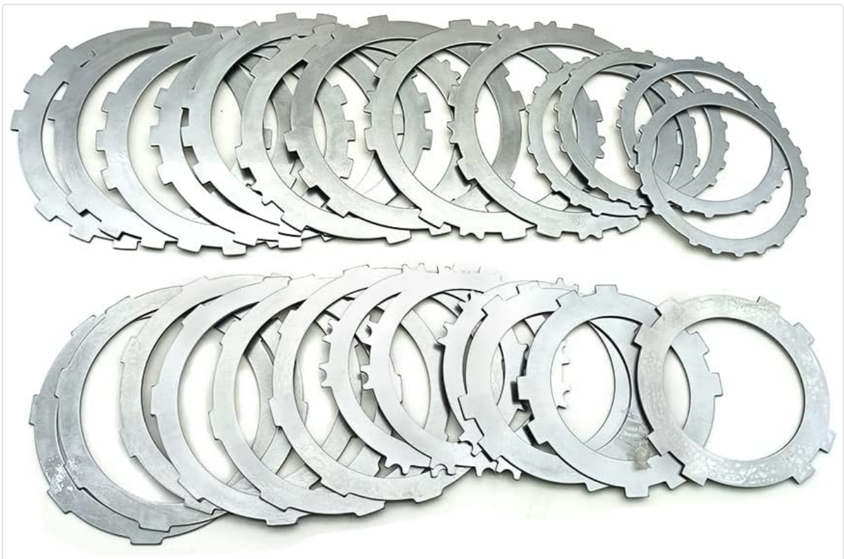
Figure 2.4: The steel plates, which work in conjunction with the friction plates to transmit power.
