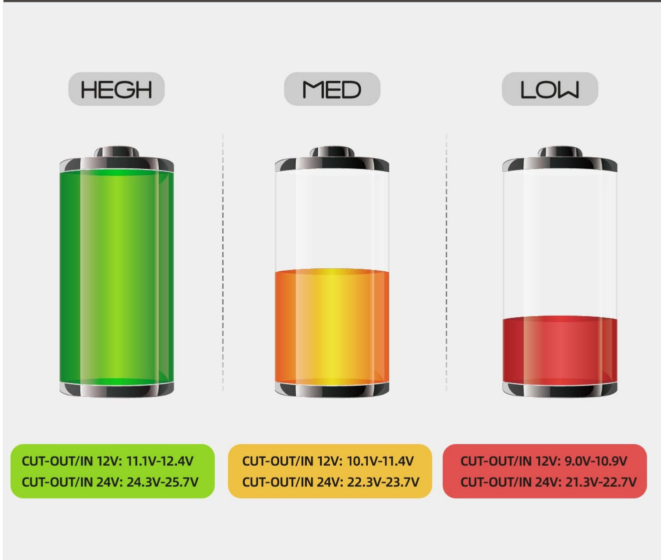
Figure 4.1: Visual representation of the three battery protection levels (High, Med, Low) and their respective cut-out voltages for both 12V and 24V power sources.
