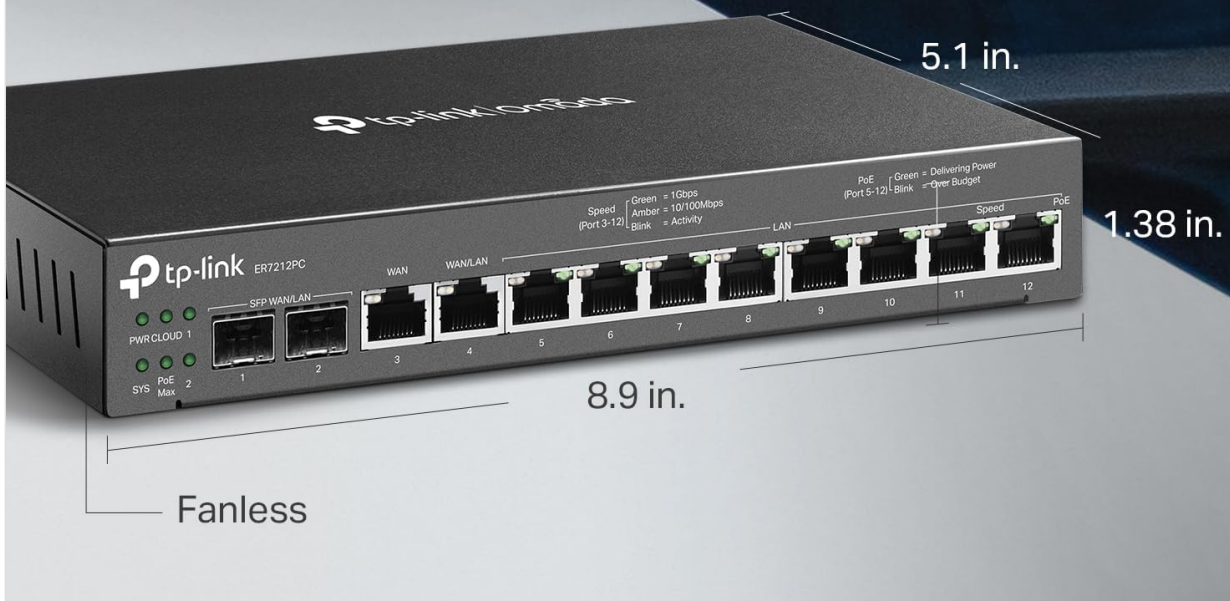
Figure 4: Compact design and fanless heat dissipation.
