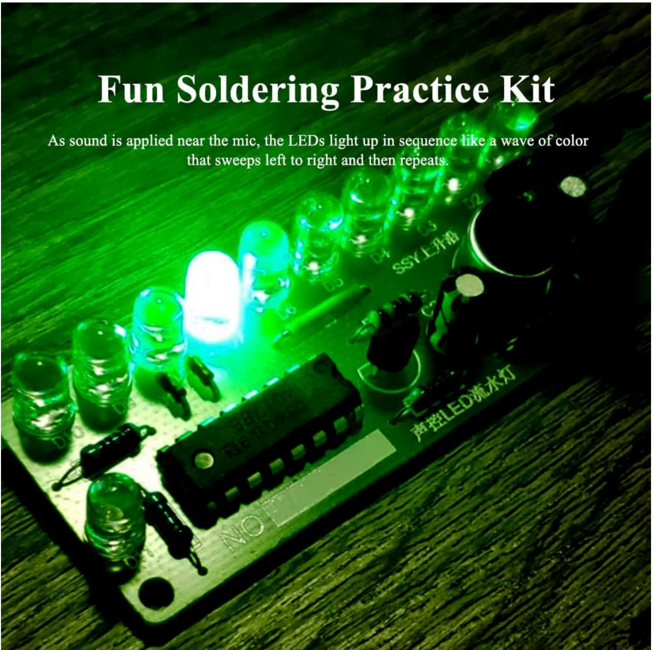
Image 6: The assembled kit demonstrating the sound-activated LED sequence.
