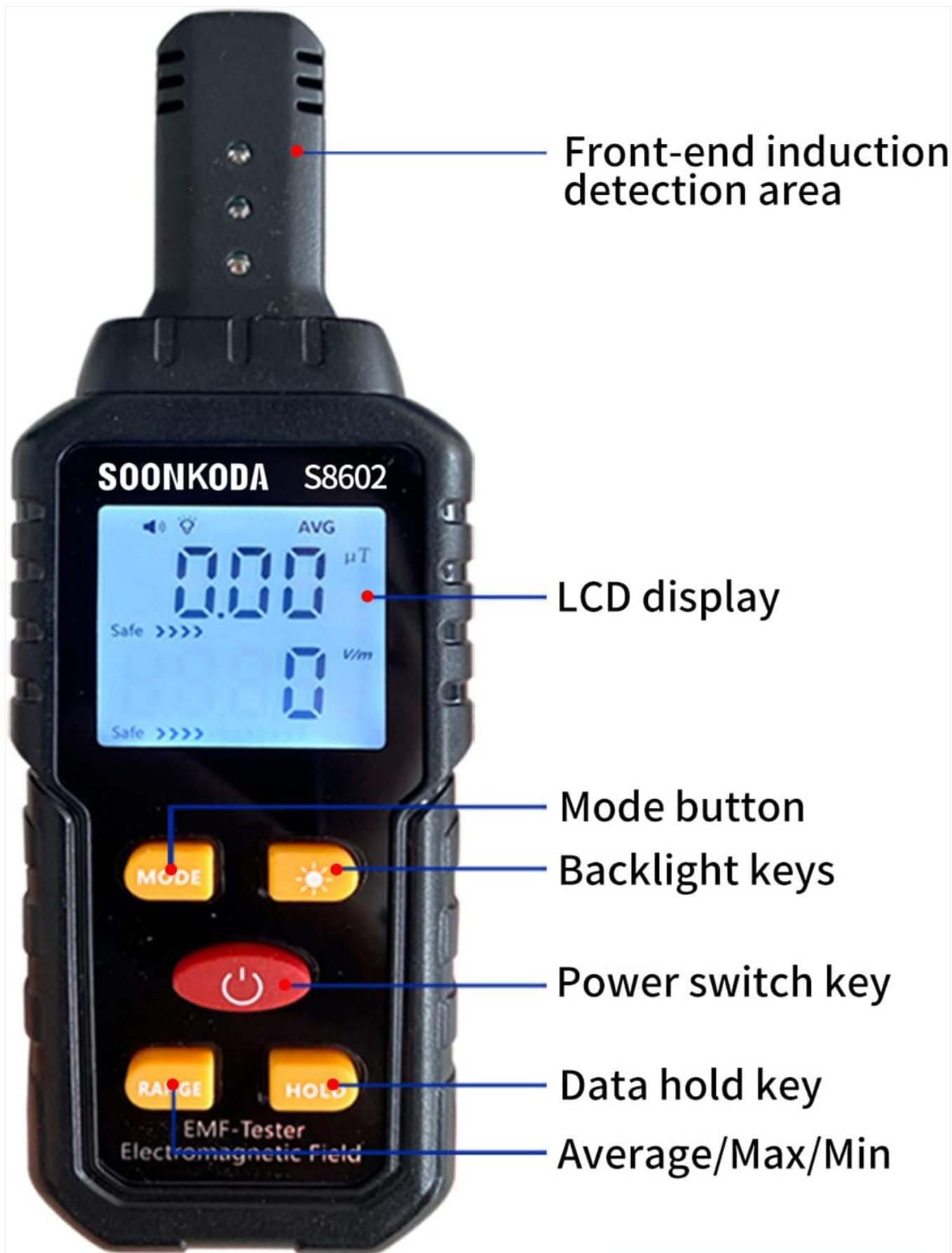
Image: Key components and controls of the Soonkoda S8602 EMF Meter.
