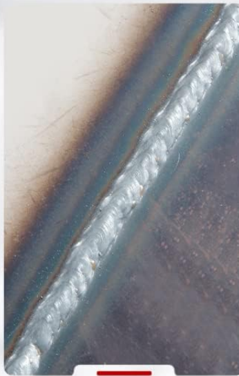
Mix Gas Welding
