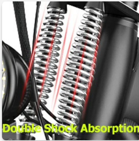
Image: A close-up view of the e-bike's double shock absorption system on the front fork, illustrating the spring mechanism for improved ride comfort.
