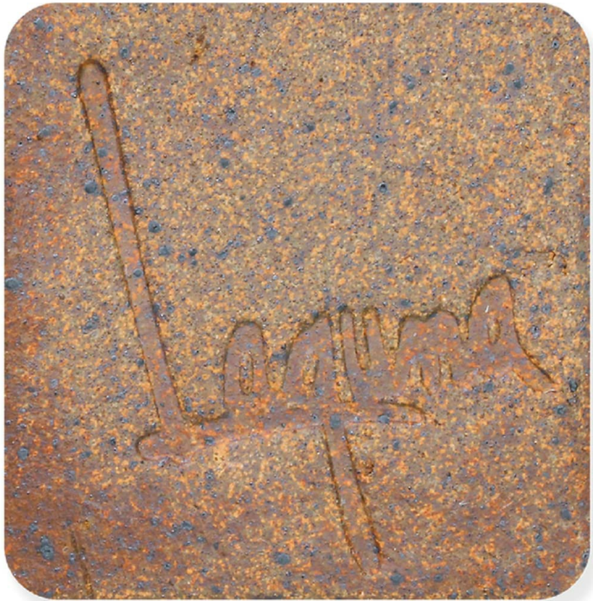
Image 1.1: Fired clay sample, demonstrating the medium brown color and iron specks achieved under reduction firing conditions.
