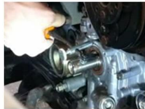
Figure 6.1: Visual guide to the seal removal process, illustrating each step from engagement to final removal.
