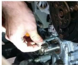
Figure 6.1: Visual guide to the seal removal process, illustrating each step from engagement to final removal.
