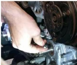
Figure 6.1: Visual guide to the seal removal process, illustrating each step from engagement to final removal.
