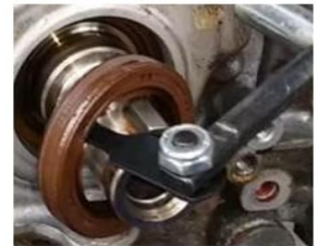
Figure 6.1: Visual guide to the seal removal process, illustrating each step from engagement to final removal.
