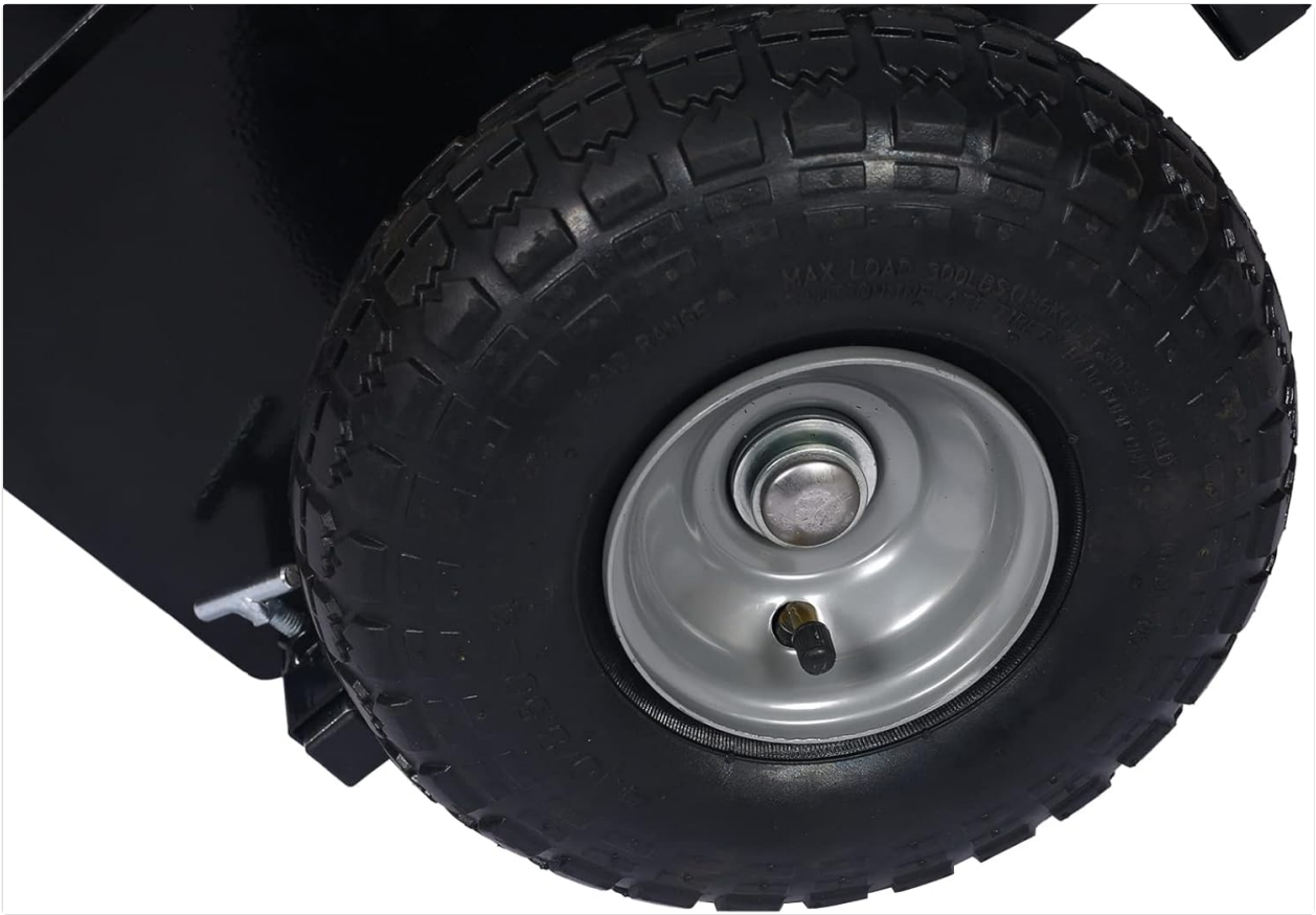
Image 5.1: A detailed view of the pneumatic wheel, showing the tire tread and valve stem for inflation.
