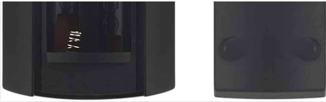
Image 2.1: The back of the remote control with the battery cover removed, illustrating the correct placement for two AAA batteries.
