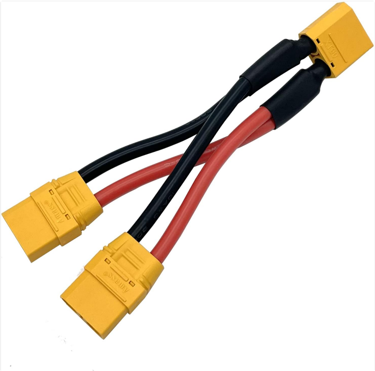
Figure 1: Overall view of the Nuofany XT90H Parallel Battery Connector Cable. This image displays the cable with one male XT90 connector splitting into two female XT90 connectors, featuring red and black 10AWG silicone wires.
