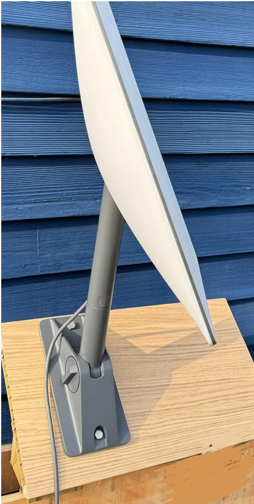
Figure 3: The Starlink Square Dish securely attached to the pivot mount, illustrating the upward angle capability.
