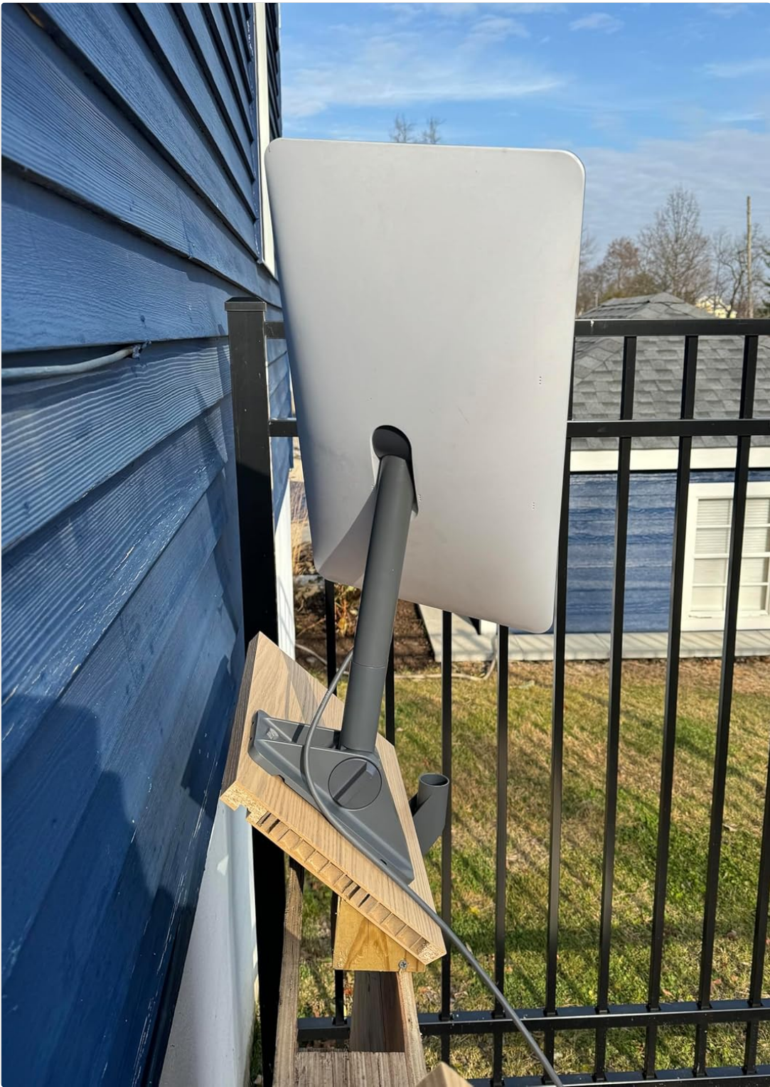
Figure 2: Example of the Starlink Pivot Mount installed on a vertical surface, demonstrating how the dish can be angled for optimal positioning.
