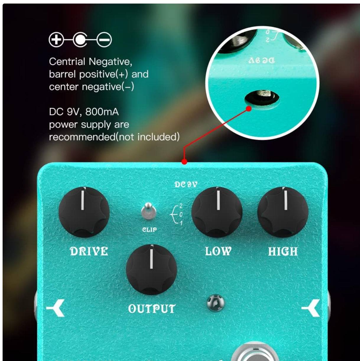
Image: Close-up of the JOYO D50 pedal's DC 9V power input jack, illustrating the required central negative polarity and power specifications.
