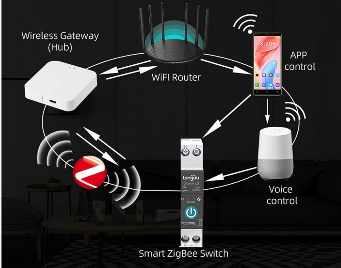
Figure 7: Diagram illustrating the connection of the Smart Zigbee Switch to a Wireless Gateway (Hub), WiFi Router, and control via APP and Voice.
