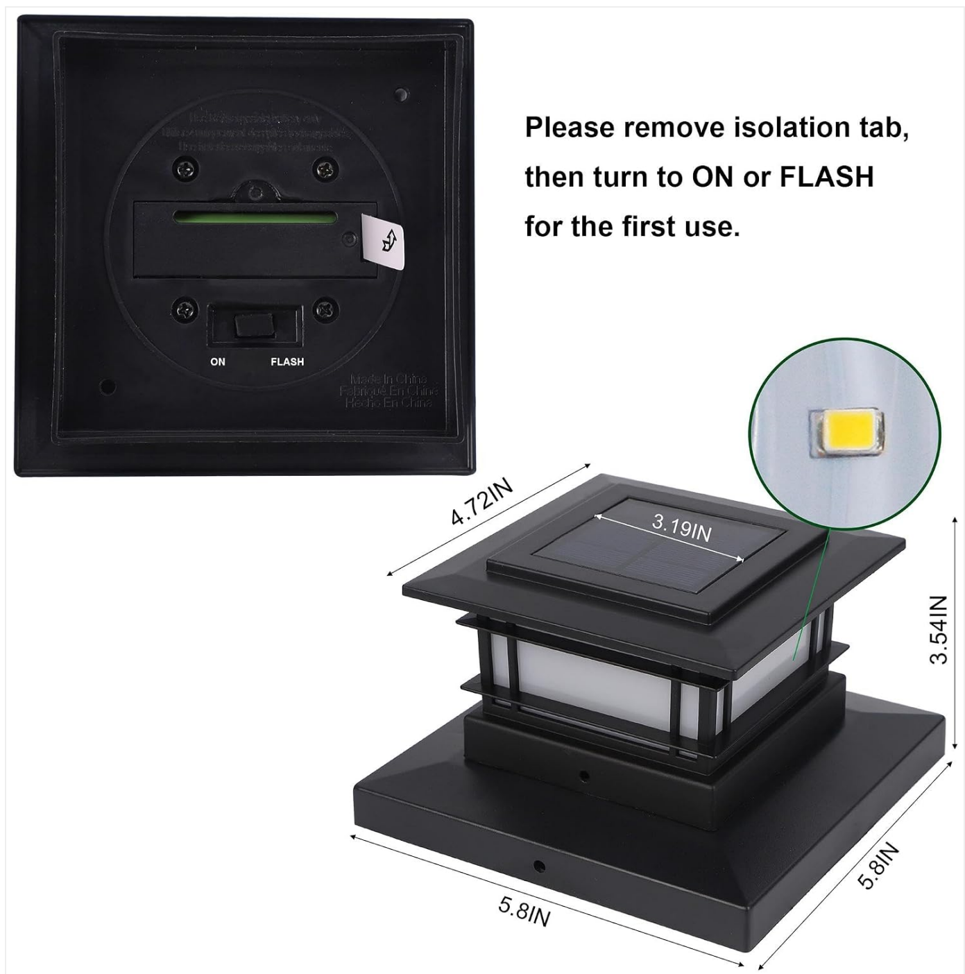
Figure 2: Underside view of the solar light, highlighting the ON/FLASH switch and the isolation tab to be removed before initial use. Product dimensions are also shown.
