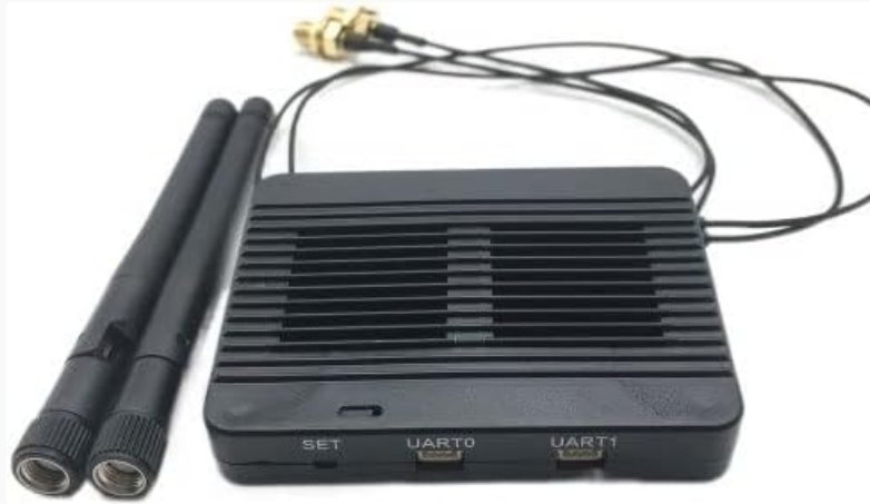
Figure 3.1: ABZEKH Skydroid H16/R16 Transmitter Unit. This image displays the main transmitter unit, a black rectangular device with cooling fins, two UART ports (UART0, UART1), a 'SET' button, and two detachable antennas connected via coaxial cables.
