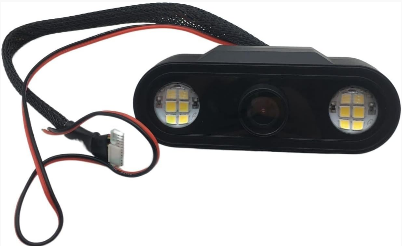
Figure 3.2: ABZEKH MIPI Camera Module. This image shows the compact black camera unit with a central lens and two integrated LED searchlights on either side. A braided cable with red and black wires extends from the module, terminating in a connector.
