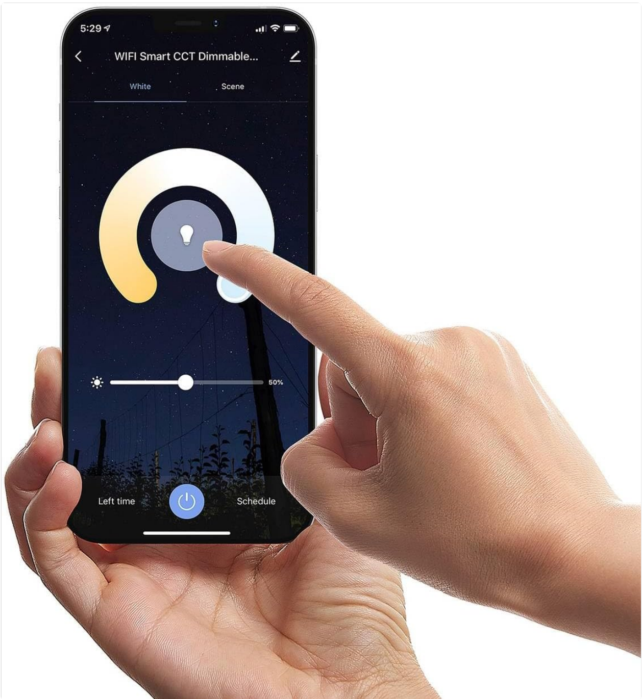
Image: A hand interacting with a smartphone displaying the Tuya app, demonstrating the light control interface for brightness and color temperature.
