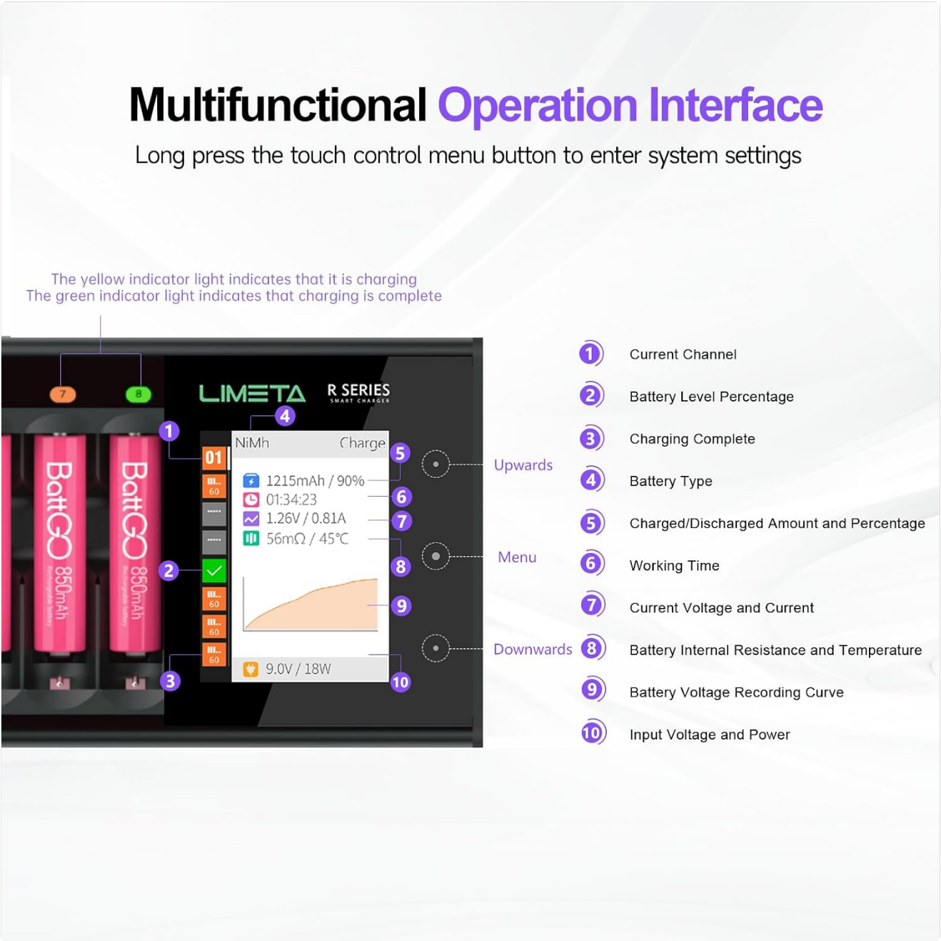
Figure 3: Multifunctional Operation Interface. The display shows current channel, battery level percentage, charging complete status, battery type, charged/discharged amount and percentage, working time, current voltage and current, battery internal resistance and temperature, battery voltage recording curve, and input voltage and power.
