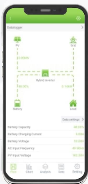
Figure 8: Illustration of the optional WiFi communication module for remote monitoring and control.
