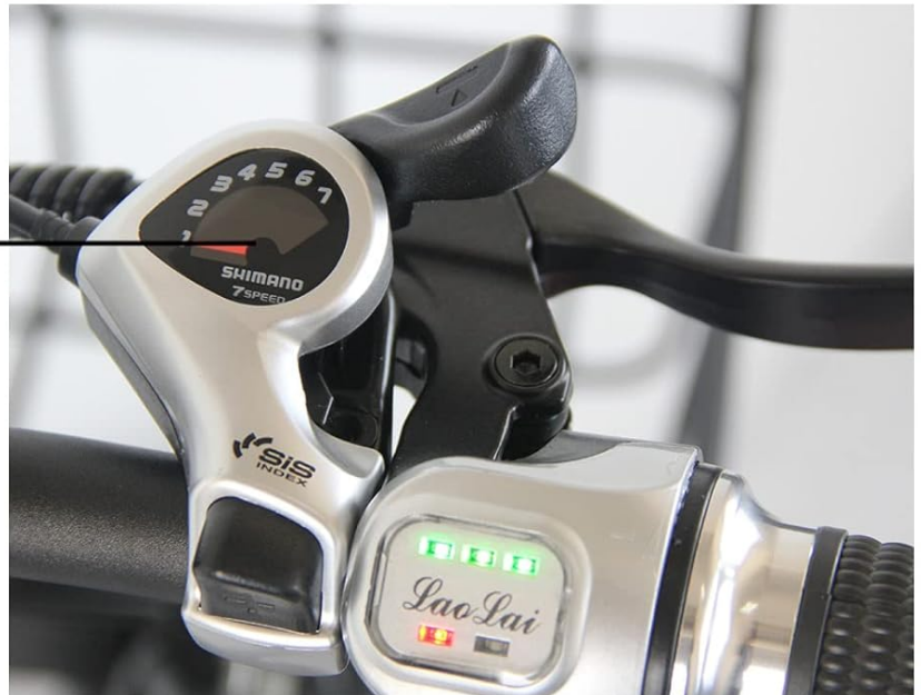
Figure 4: Intelligent Liquid Crystal Instrument and Shimano TX50 Shifter. This image highlights the digital display showing speed and battery, and the 7-speed Shimano shift lever for gear changes.
