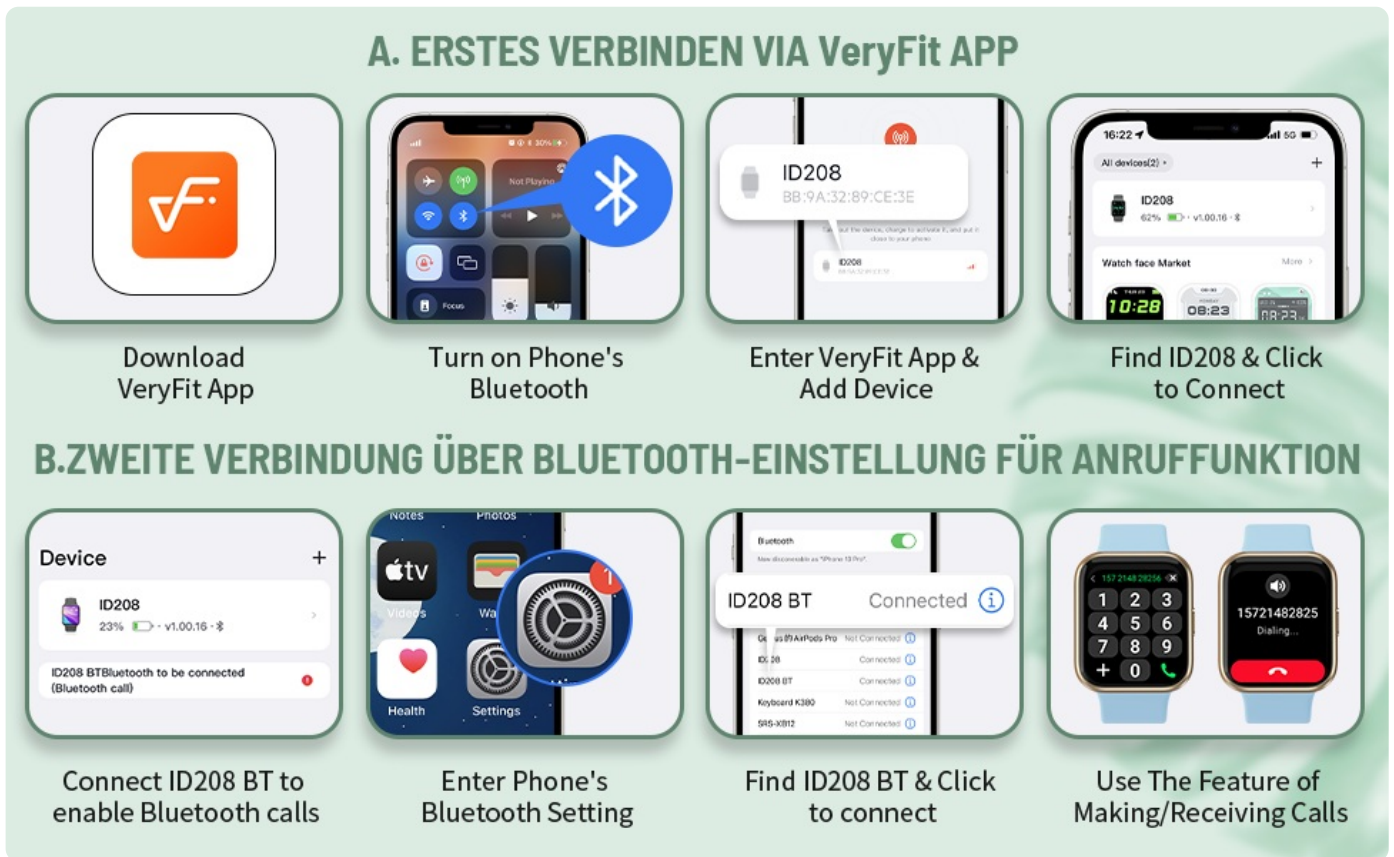
Image 3.2: App and Bluetooth Call Connection Steps. This image provides a visual guide for connecting the smart watch to the VeryFit app and subsequently enabling the Bluetooth call feature through the phone's Bluetooth settings.
