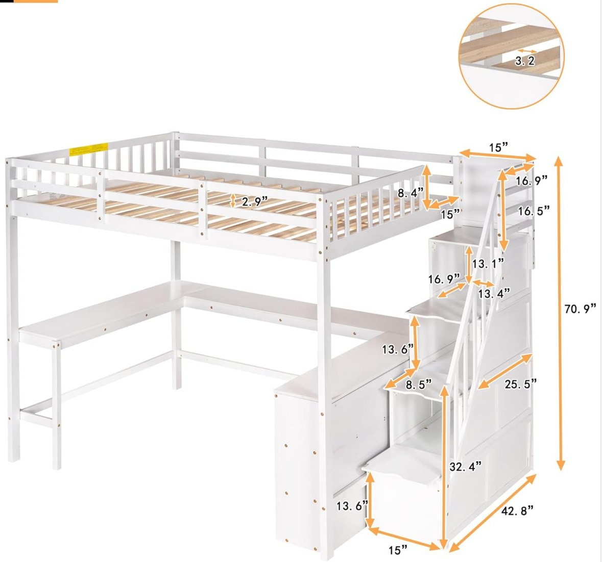
Image: Dimensional drawing of the loft bed, providing precise measurements for all sections.
