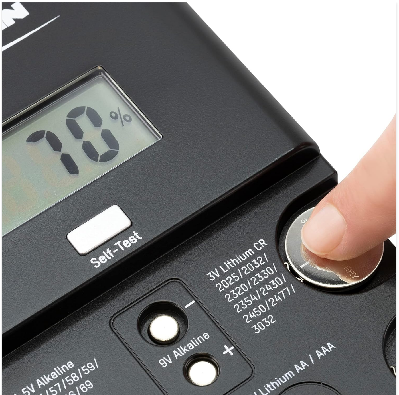
Figure 5: Testing a Button Cell Battery. This image shows a user testing a small button cell battery by pressing it onto the designated contact points.
