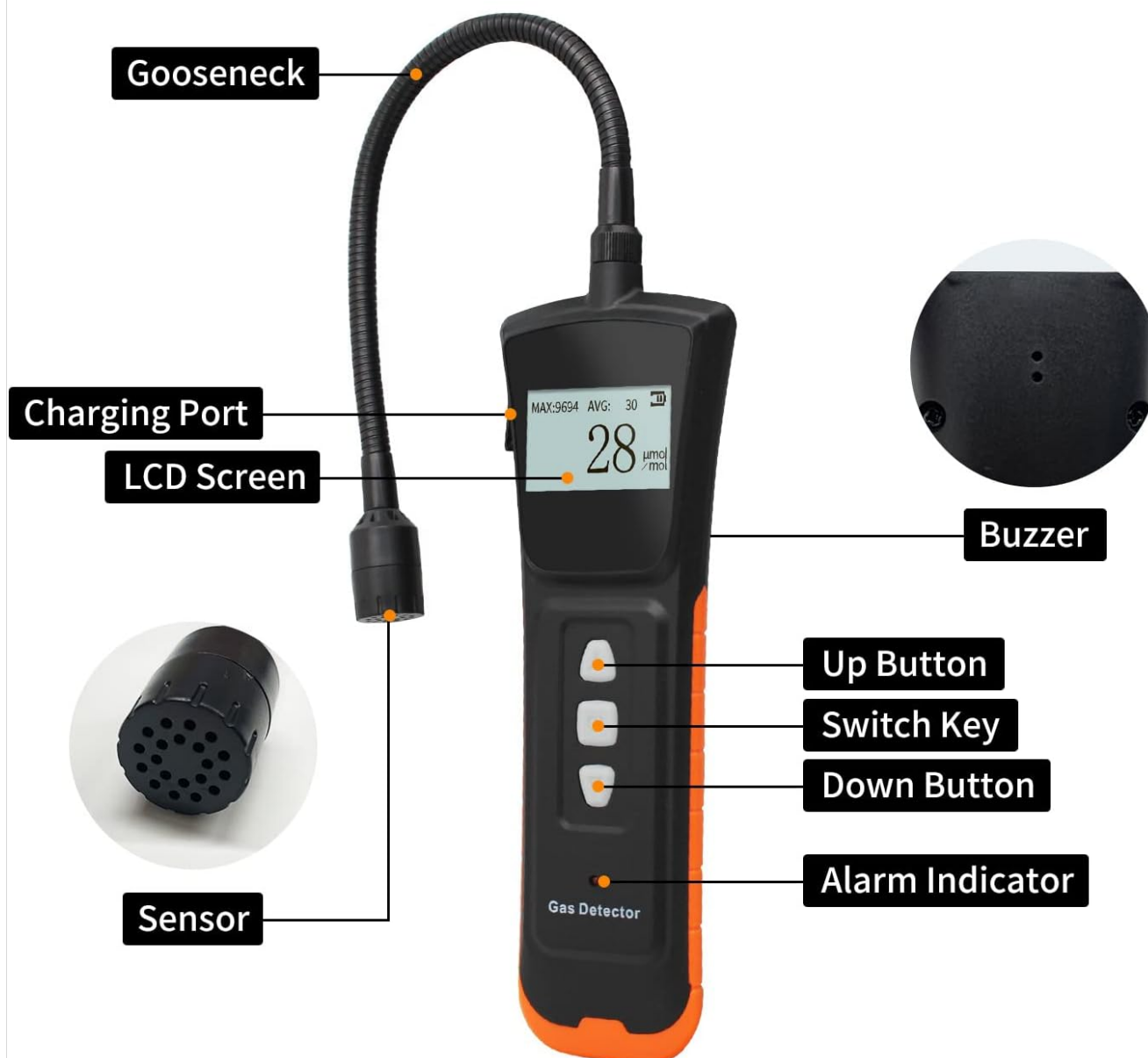
Image: Detailed diagram labeling the various parts of the CHNADKS Gas Leak Detector.
