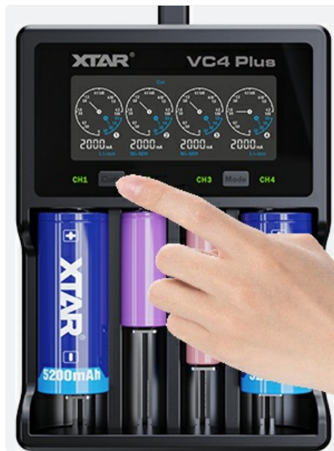
Image 4: Adjusting charging current.
