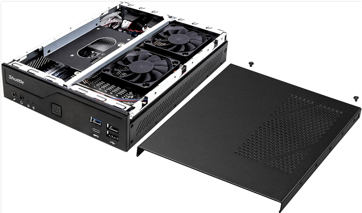
Image: The Shuttle XPC Slim DH610 with its top cover removed, showing the internal layout including cooling fans and the motherboard.
