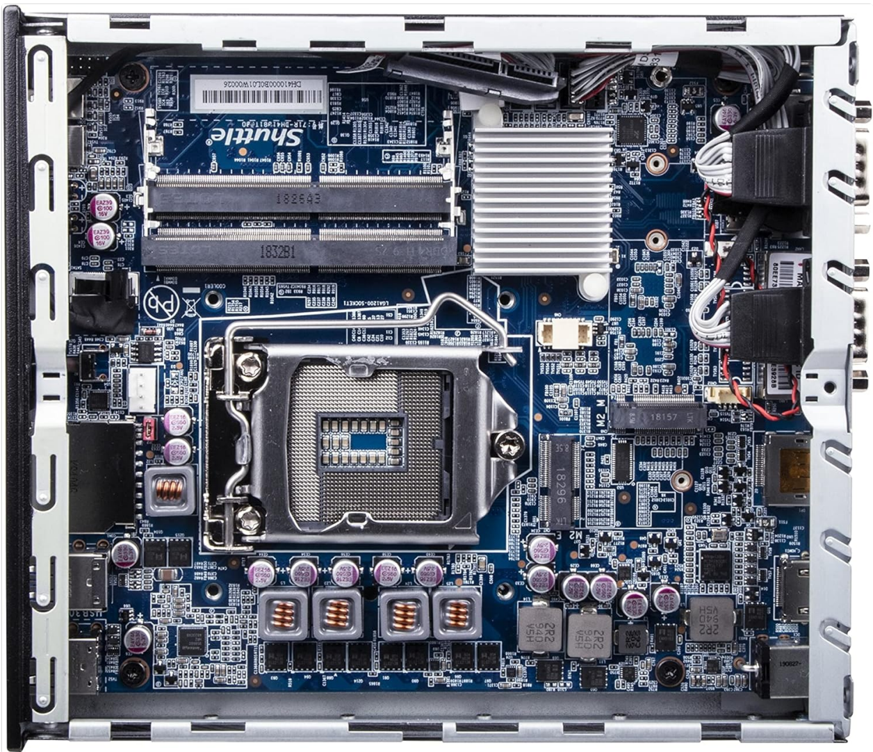
Image: A detailed view of the Shuttle DH610 motherboard, highlighting the LGA1700 CPU socket, RAM slots, and other integrated circuits.
