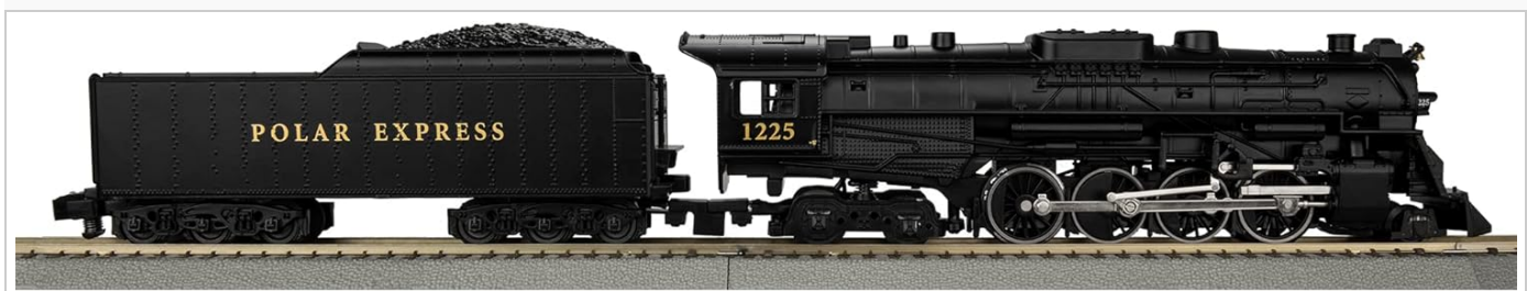
Figure 4: Side view of the 2-8-4 Berkshire steam locomotive and tender.
