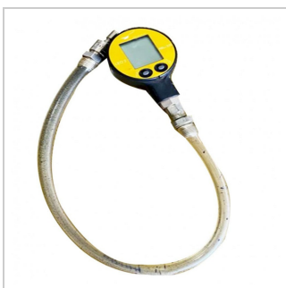
Figure 6: The LEO2 gauge connected to a flexible hose, demonstrating its adaptability for various setups.
