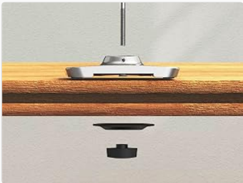
Image: Exploded view of the Grommet mounting base, illustrating how it secures through a desk hole.
