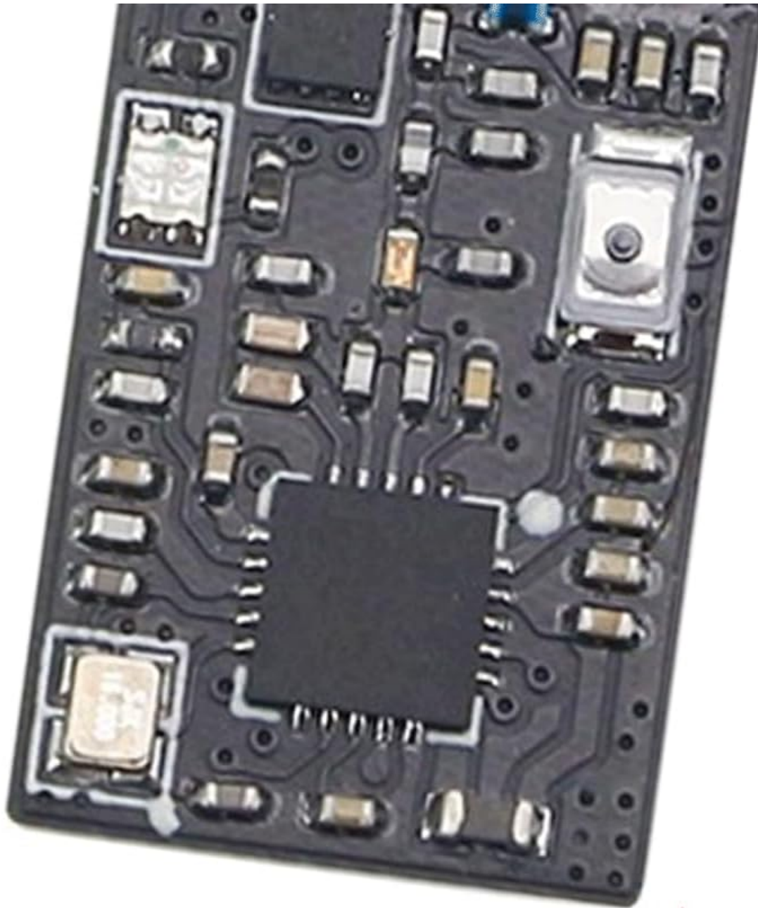
Image: The LDARC X-BOSS FM900 receiver, a compact circuit board featuring surface-mount components, an integrated antenna, and clearly labeled 'FM900' branding. This image illustrates the physical design and component layout of the receiver.
