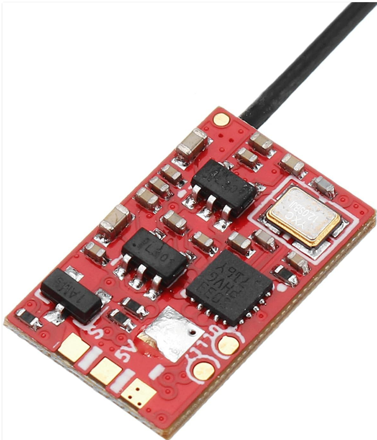
Figure 2: Close-up view of the AC900 receiver's components, highlighting its compact design.
