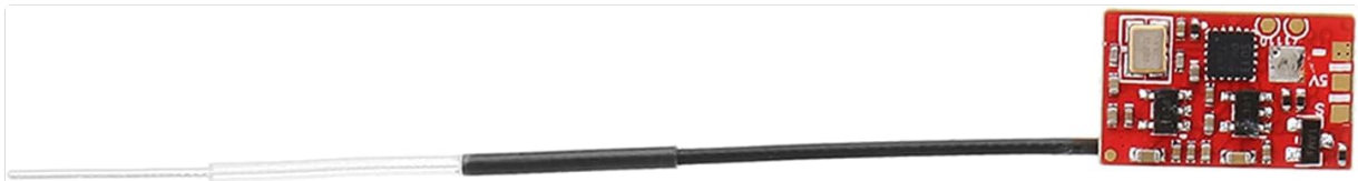
Figure 1: Top-down view of the LDARC X-BOSS AC900 receiver, showing its compact size and integrated antenna.
