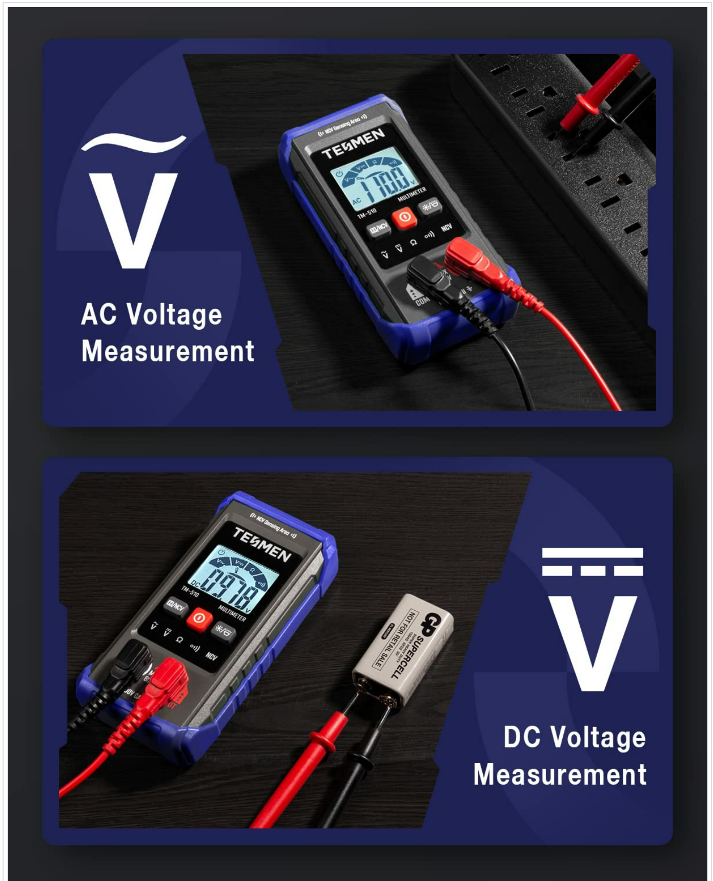
Figure 5.3: The multimeter measuring AC voltage from a power strip (top) and DC voltage from a 9V battery (bottom).
