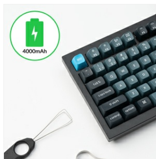
Image 3.1: The Keychron Q1 Pro features a 4000mAh battery for extended wireless use.
