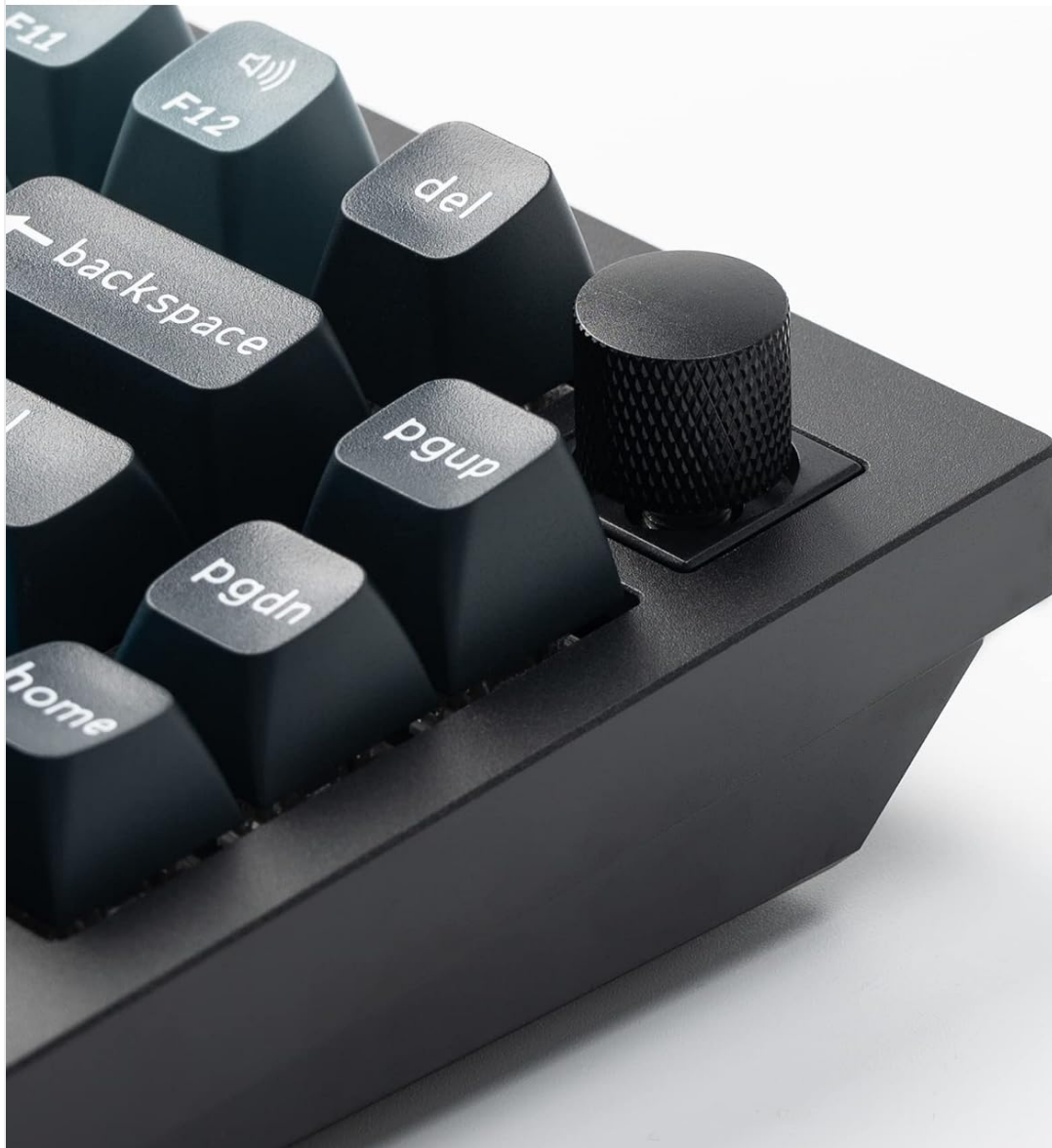
Image 4.3: The programmable knob offers quick access to customizable functions.
