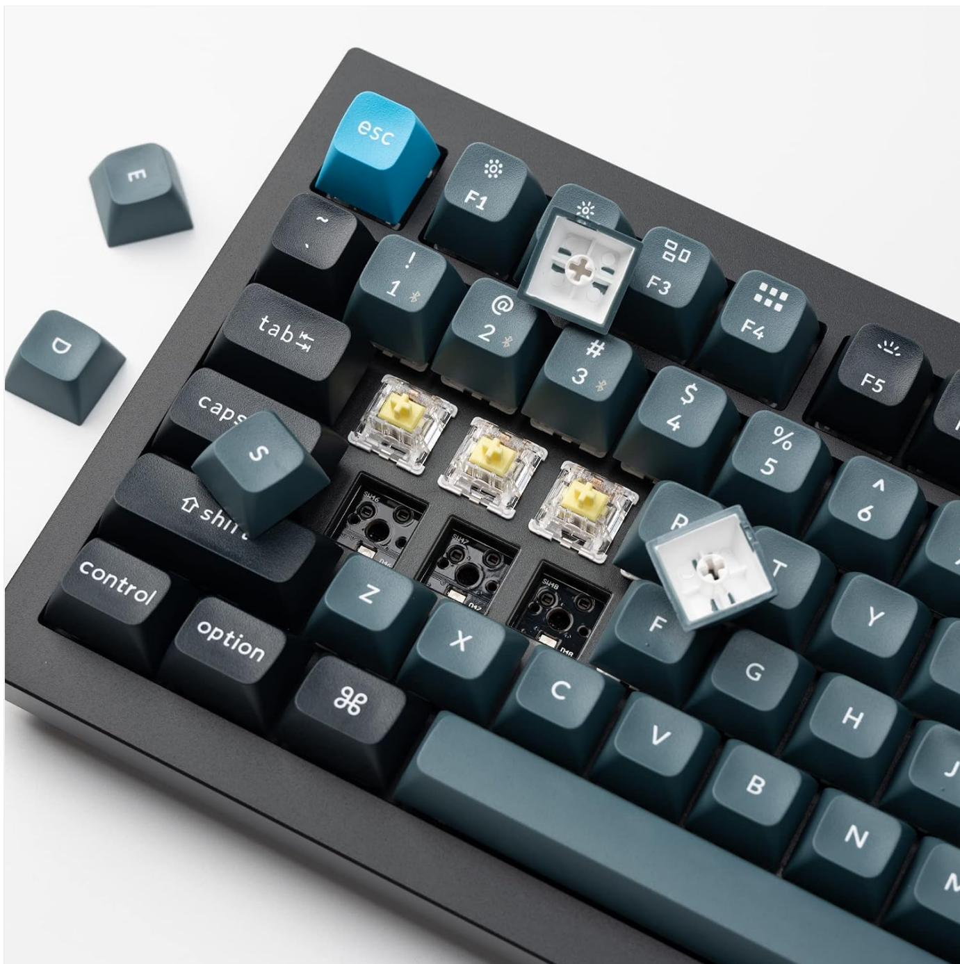
Image 5.2: Demonstrating the hot-swappable feature by removing keycaps and switches.
