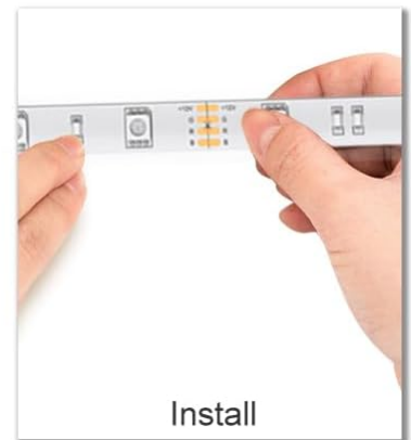
Figure 4.3: Strip Application - Apply pressure evenly to ensure good contact with the surface.
