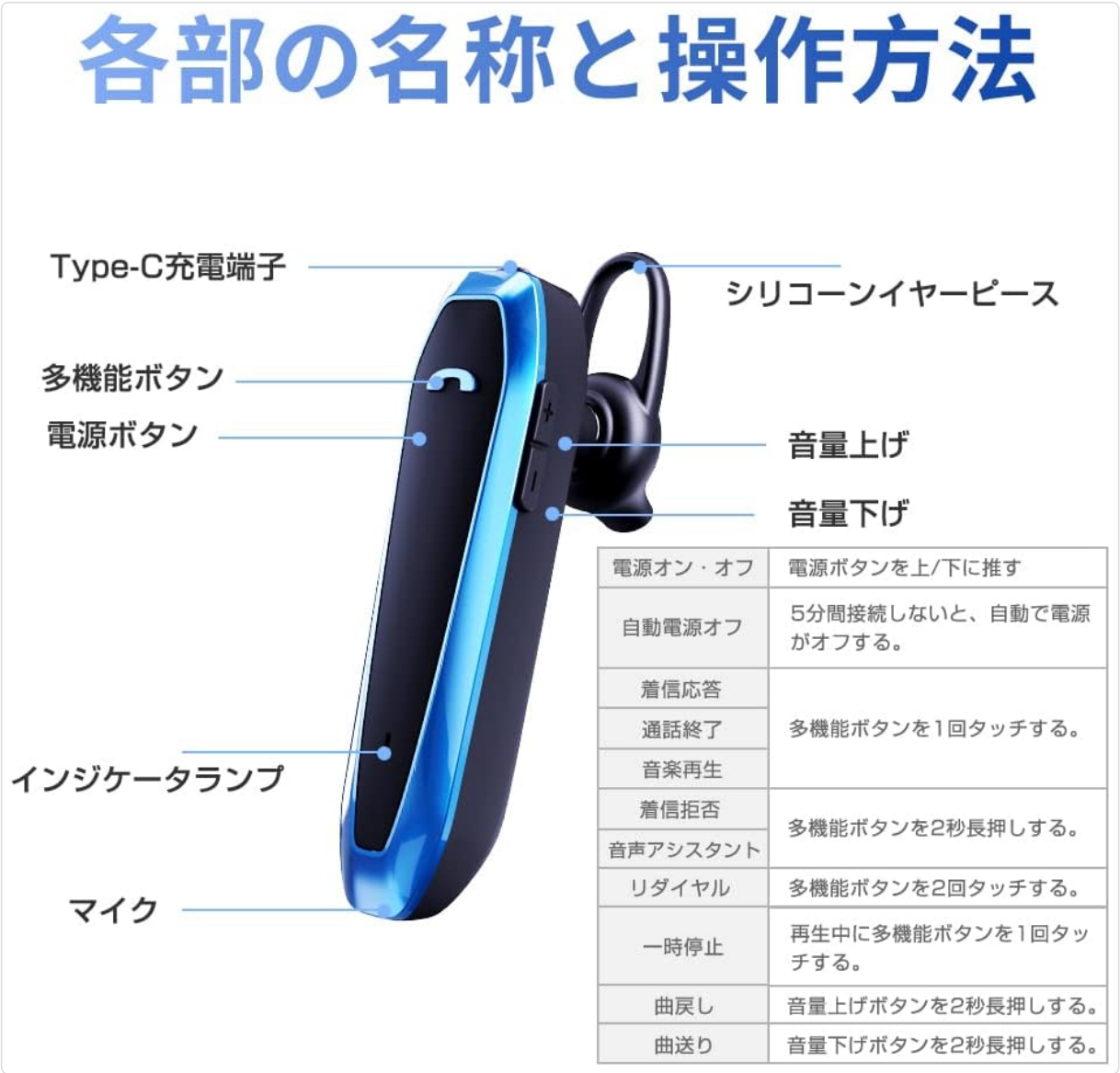
Image 3.1: Headset Components and Controls. This diagram illustrates the location of the Type-C charging port, multi-function button, power button, volume up/down buttons, indicator lamp, microphone, and silicone earpiece.
