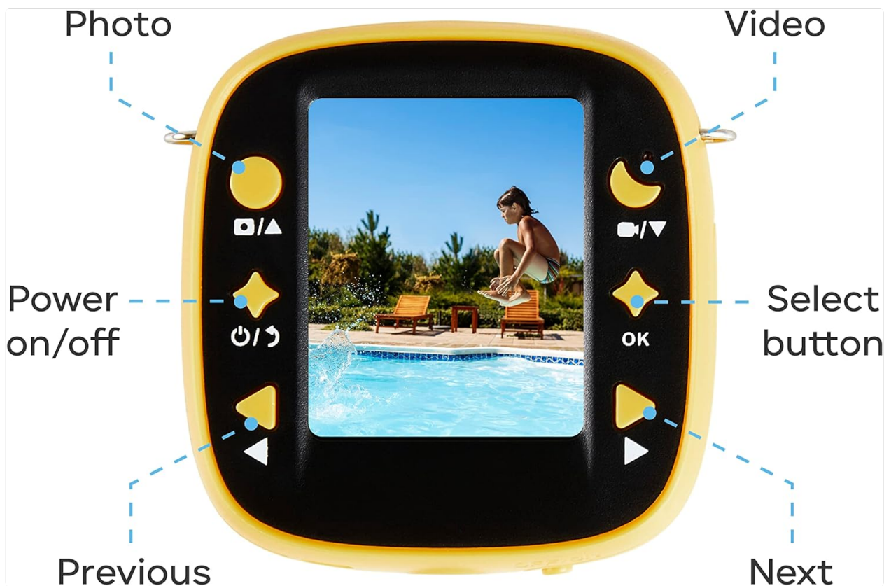
Figure 3: Detailed view of the camera's rear, indicating the Photo, Video, Power On/Off, Select, OK, Previous, and Next buttons around the display.
