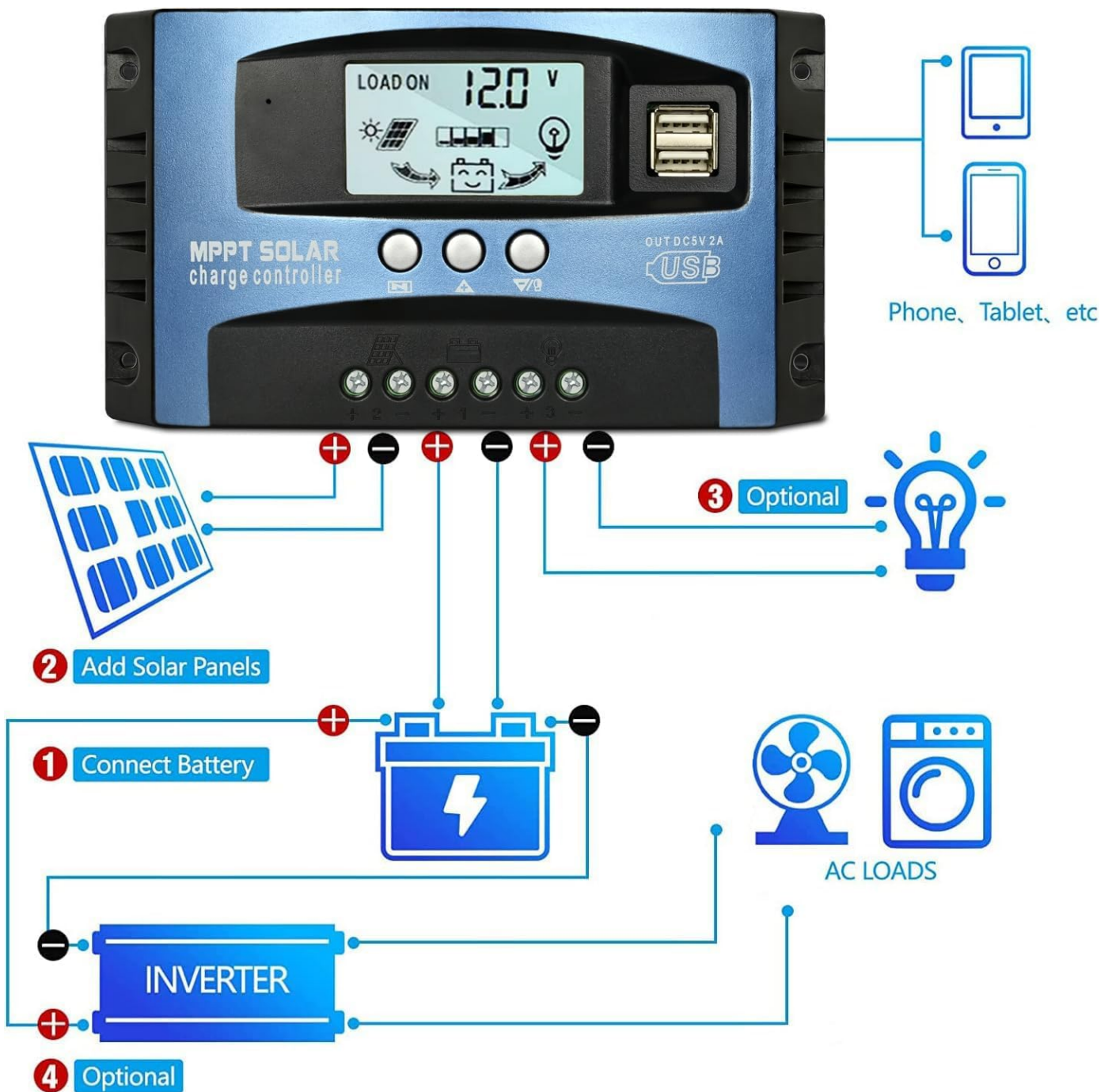
Image: Detailed wiring diagram illustrating connections for the battery, solar panels, and optional inverter/load.
