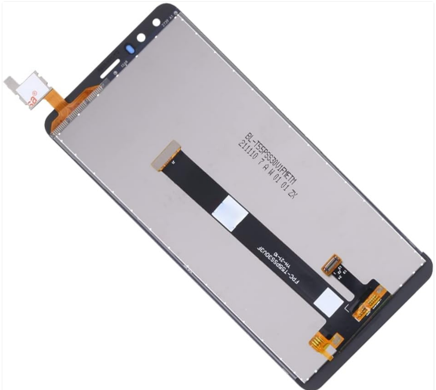
Image: The reverse side of the replacement LCD screen, showing the delicate flex cables that connect to the phone's motherboard.
