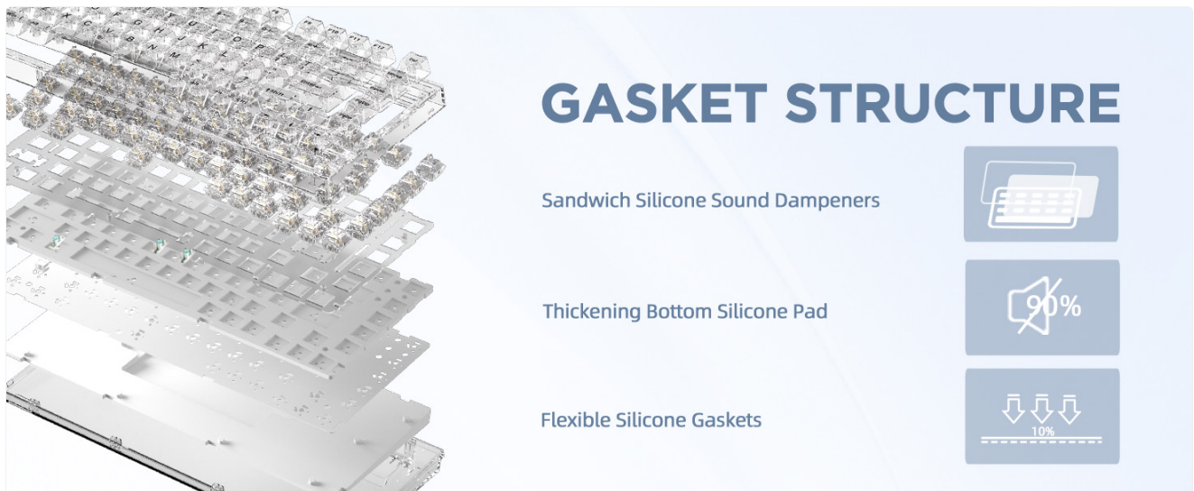
Image 3.2: Detailed view of the gasket structure.
